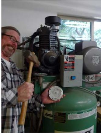
sity. With that there said, one of my personal pet peeves is the steady hissing sound of air leaks. I can't handle that and I will not have it. As of late I've noticed that our air supply leaks down some overnight, even with the main ball valve closed. Our compressor owes us nothing and deserves a little love. Perhaps it's time to have a look inside its automatic drain valve.
